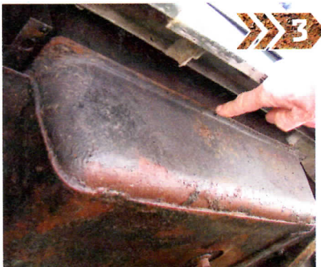
Series III short-wheelbase fuel tanks corrode along this seam and also at the attachment points of their mounting brackets
