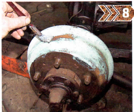
Brake drums can rust heavily but rarely become weakened. For looks, apply rust converter and a heatproof top coat
