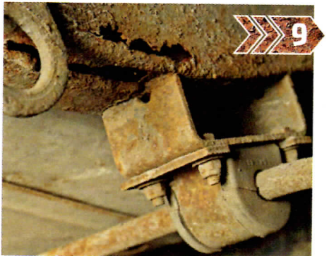
The Defender's main chassis rails often corrode through around the rear-anti-roll bar-to-chassis mounting brackets
