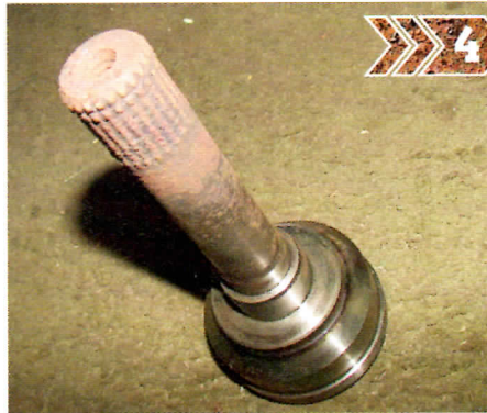
Rusting can lead to failure of the outer axle shaft splines. Keep them lightly greased if you're frequently driving through water
