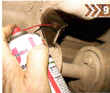
Underbody rust protection on later Land Rovers is excellent. But oil Freelander 1 prop bearing bolts to prevent them from rusting in
