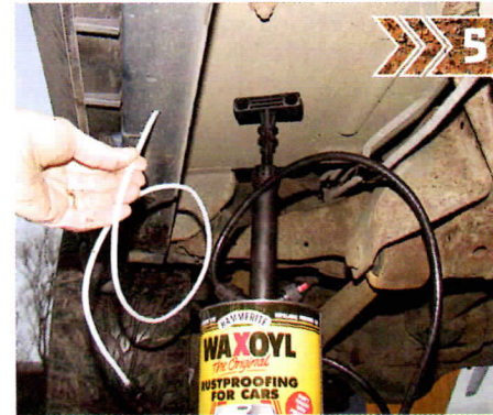
Waxoyl and Dinitrol add more external protection. It's also ideal inside chassis, bulkhead, and these Disco sills
