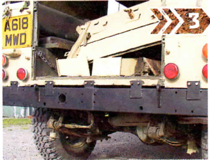
No matter how well prepared and painted, a new chassis section will need an annual check and touch-up to keep it rust-free
