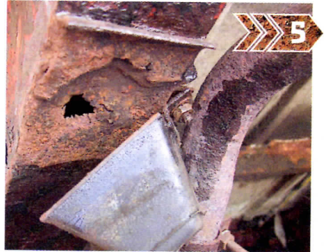
When rustproofing the chassis, remove the suspension bumps stops to treat the hidden steelwork behind them
