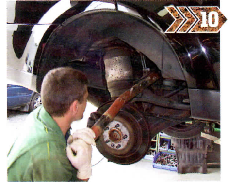
Apply anti-seize grease to bolt threads. It avoids needing a 2ft pipe to release a rusted bolt, as on this new-ish Range Rover Sport
