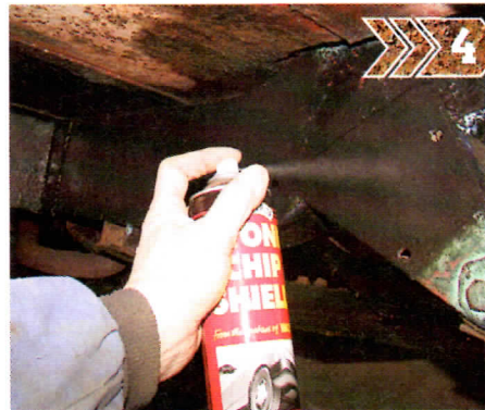
My choice is stone chip paint: it's tough, flexible, looks neat and is easily touched up during the annual paint check
