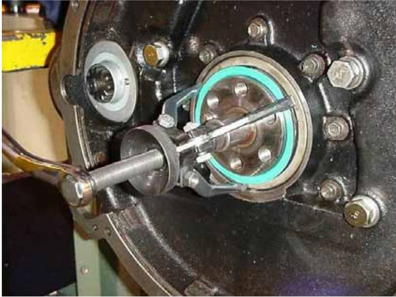
**Figure 39 Removing the New Type of Oil Seal**
