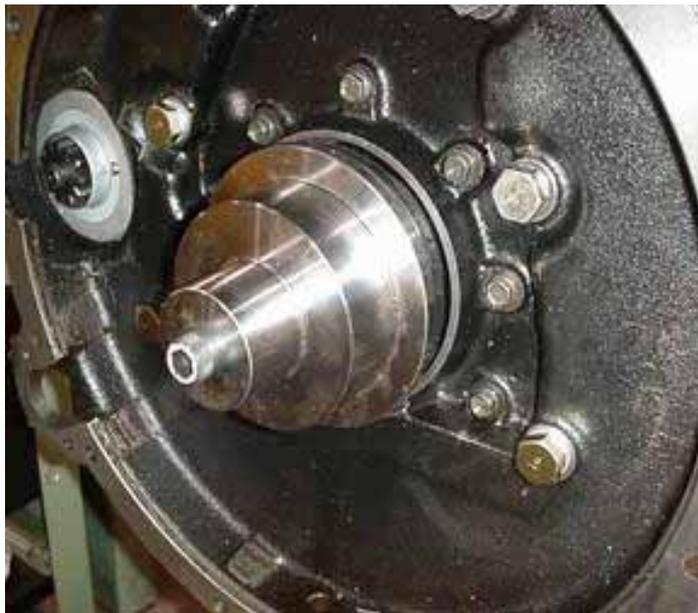
Figure 42 Push Cone (Located on Crank Plate and Against the Seal)
