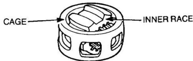
**Figure 278 Removal of the Inner Race**
