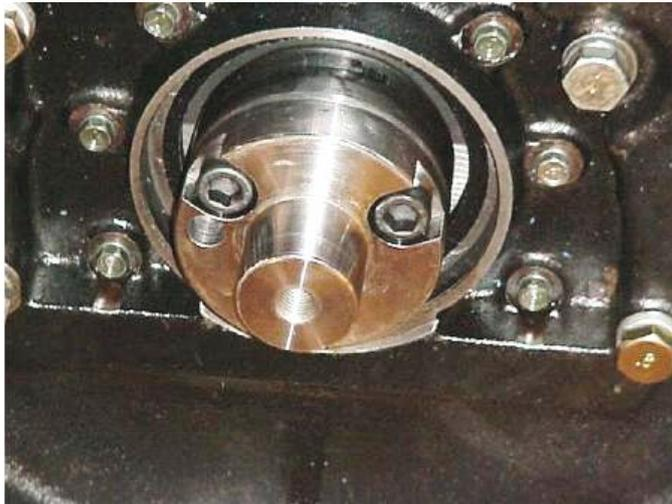
**Figure 48 Crank Plate Secured to the Crankshaft**
