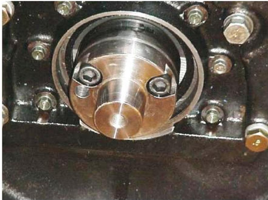
**Figure 48 Crank Plate (Secured to Crankshaft)**
