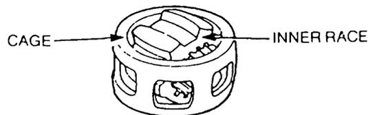
**Figure 121 Inner Race Removal**
