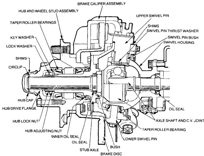
Figure 54 Steerable Drive-end – Sectional View
