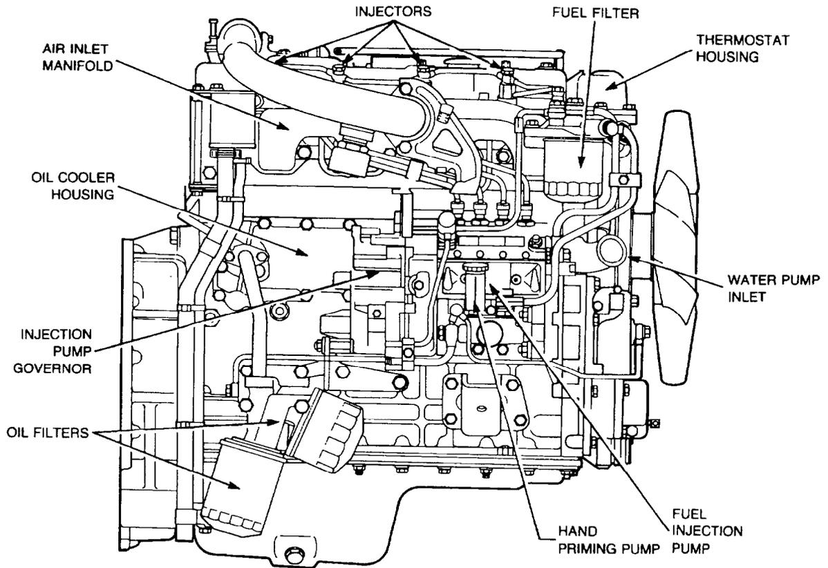
Figure 3 Isuzu Engine 4BDT1, Right-hand Side
