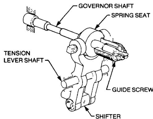
Figure 27 Tension Lever and Governor Shaft
