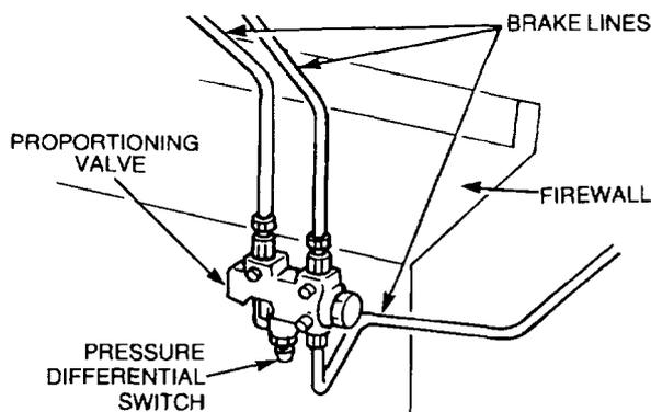
**Figure 56 Pressure Differential Switch – Location**
