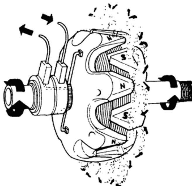
**Figure 79 Rotor and Magnetic Field**
