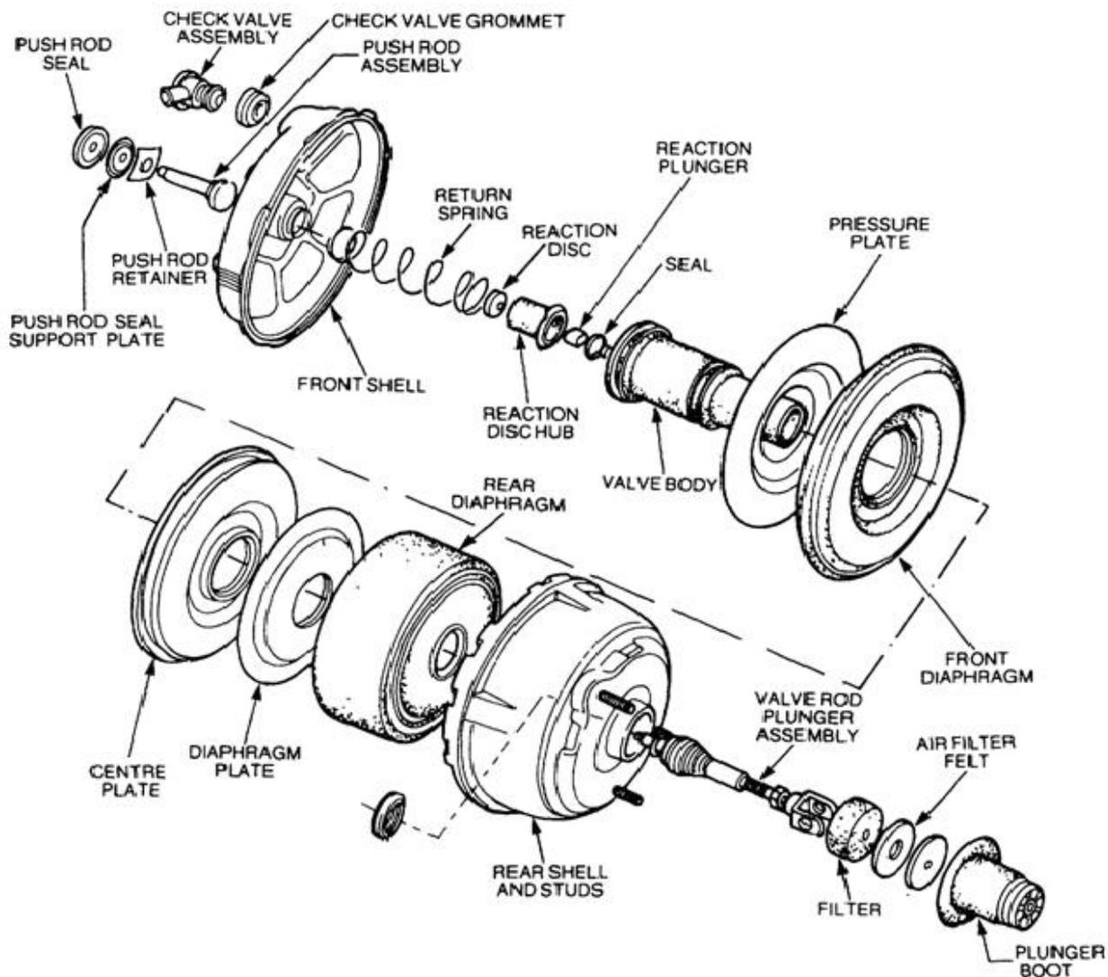
Figure 60 Brake Servo Vacuum Chamber – Exploded View
