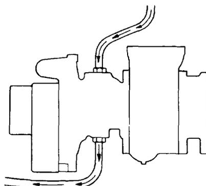
Figure 8 Cooling System – Coolant Flow
