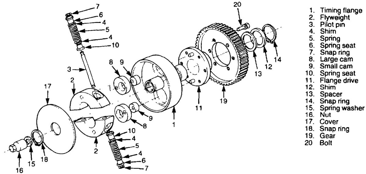
Figure 40 Automatic Timer – Exploded View
