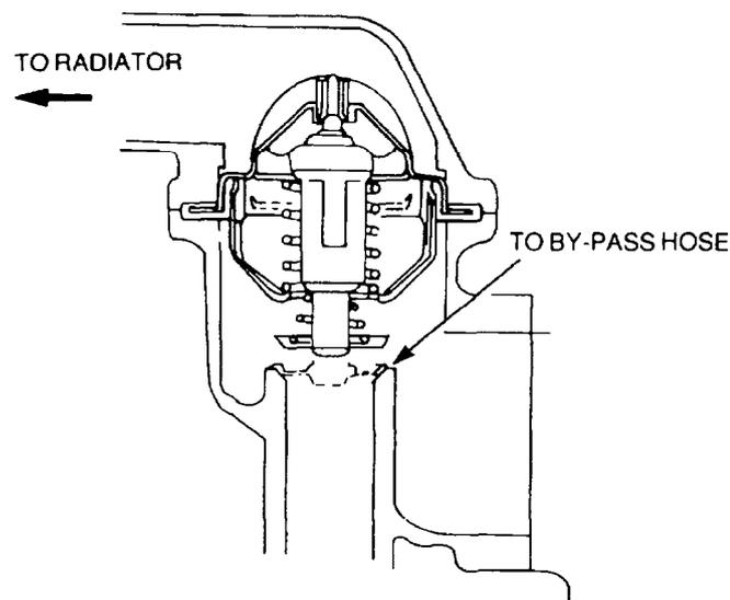
**Figure 6 Thermostat Operation**
