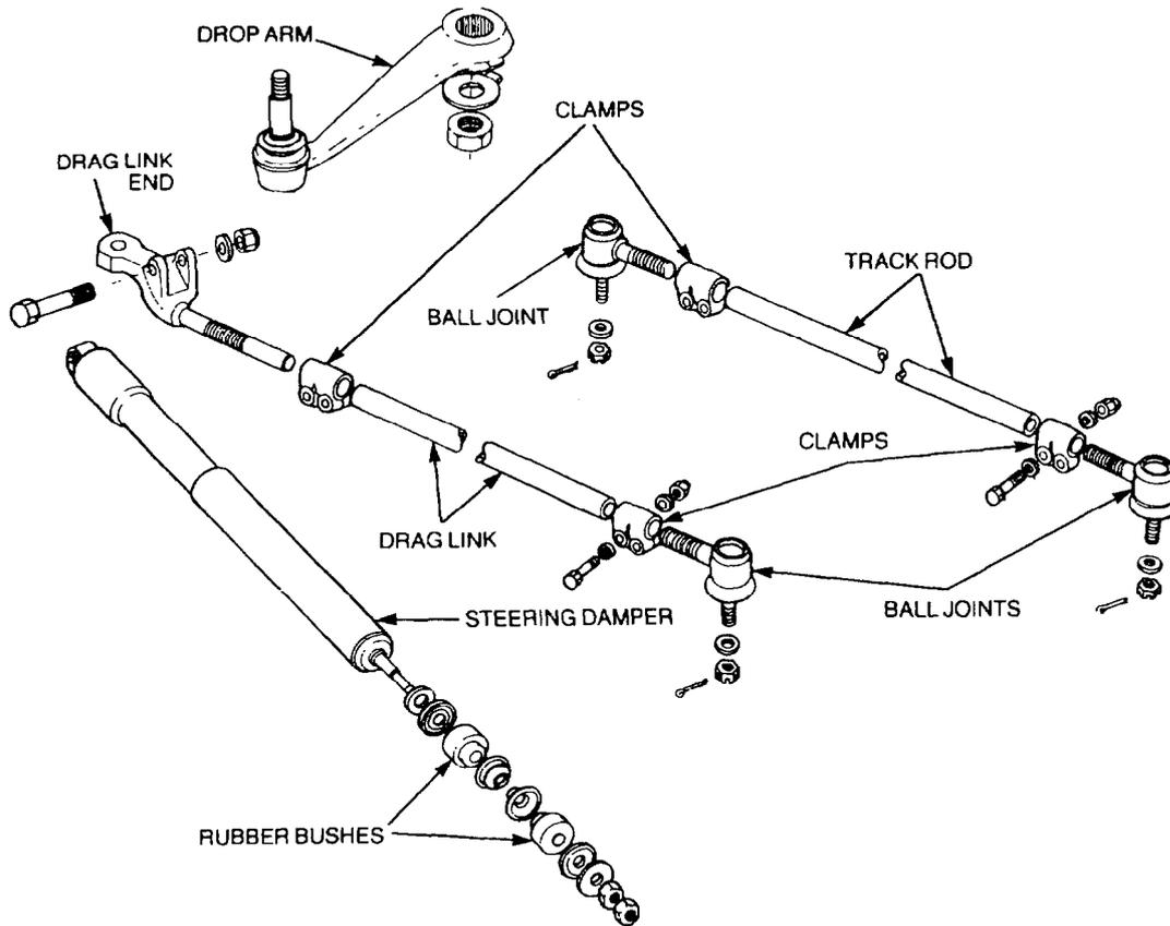
**Figure 73 Drop Arm, Steering Linkages and Steering Damper**
