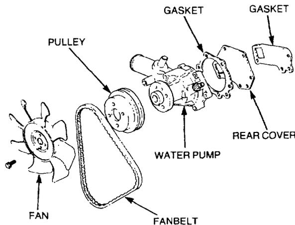
Figure 7 Water Pump Assembly
