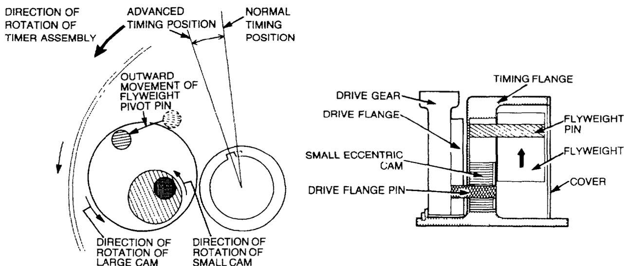
Figure 42 Flyweights in Timing Advance Position
