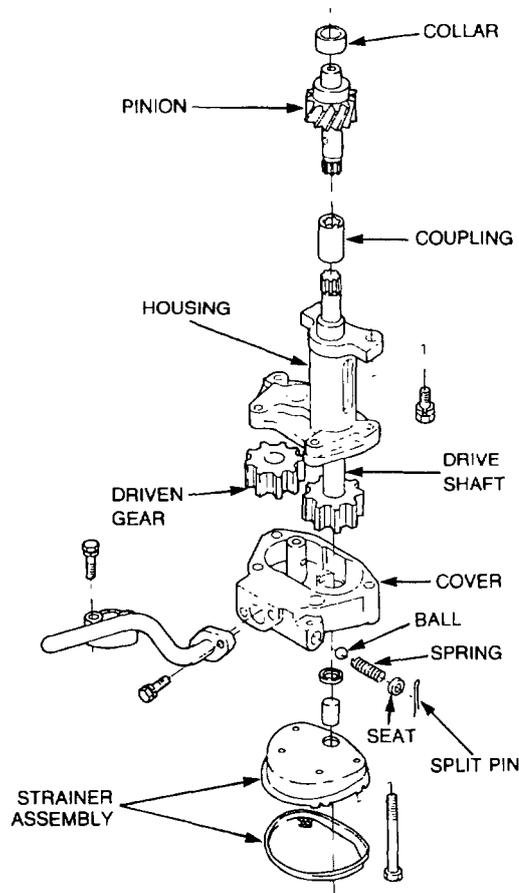
Figure 5 Oil Pump – Exploded View
