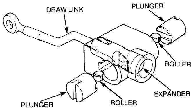
Figure 65 Parking Brake Expander Assembly – Exploded View
