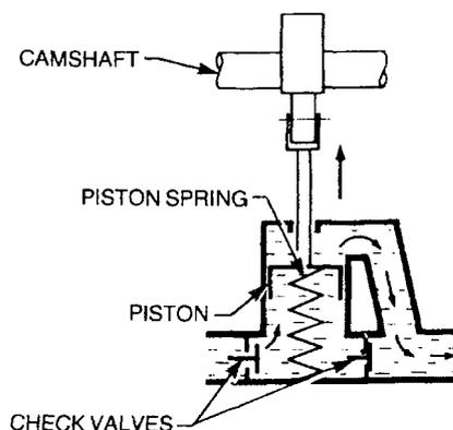
Figure 13 Intake Stroke
