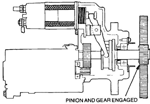
Figure 76 Ignition Switch in START
