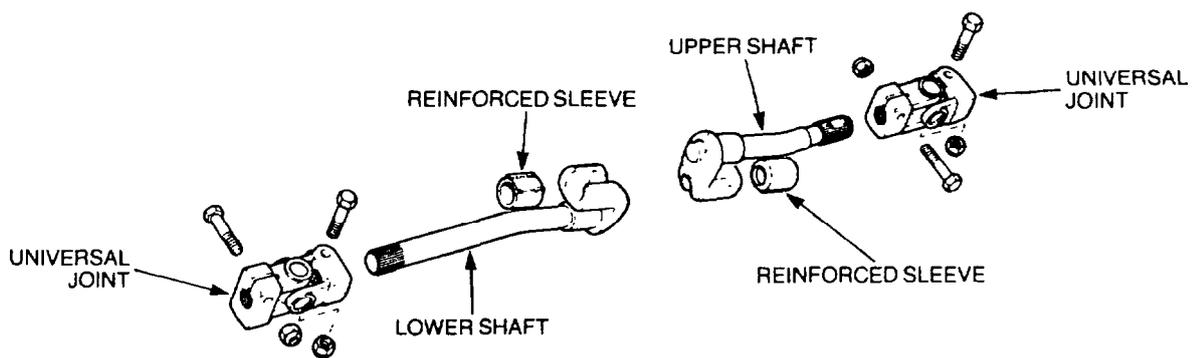
**Figure 71 Steering Shaft (Lower Section) and Coupling – Exploded View**
