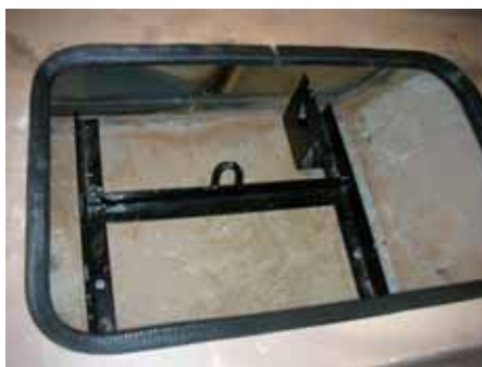
Figure 13 Orientation Of The Battery Mount Frame
