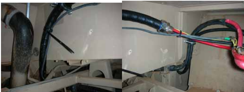
Figure 35 LH Side Crossover Harness Routing and Earth Link Connection
