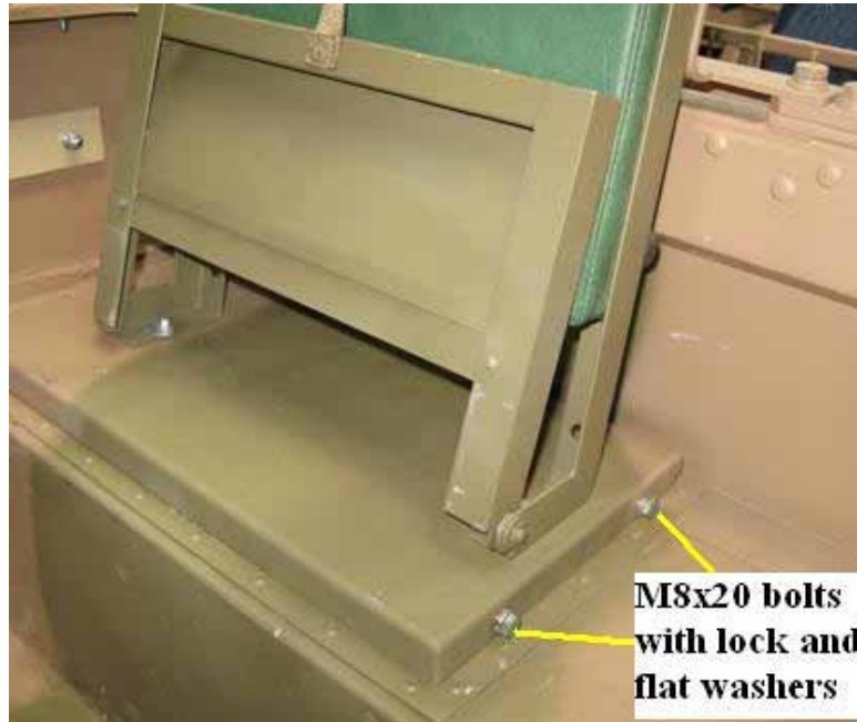
Figure 55 Main Battery Box Cover and Side-facing Seat Installed
