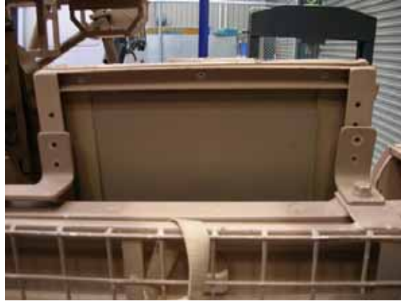
Figure 17 Position of the Holes to be Drilled Through the Upper Seat Mount Bracket
