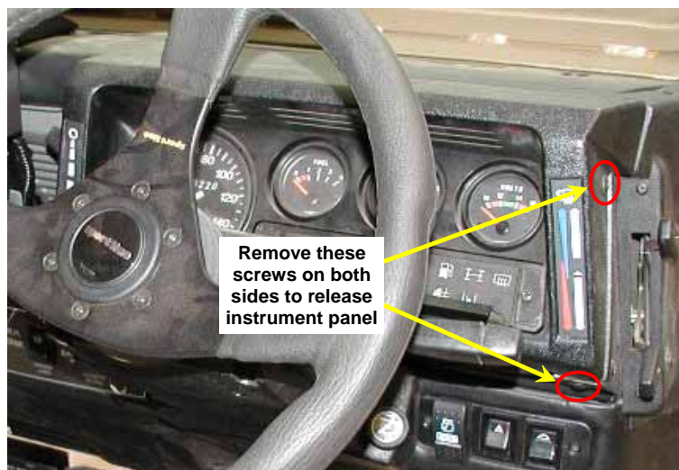
Figure 2 Instrument Panel Securing Screws
