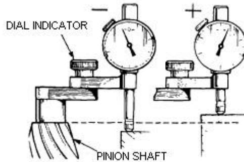
**Figure 223 Measuring the Pinion Shaft Height Using the Zeroed Dial Indicator**
