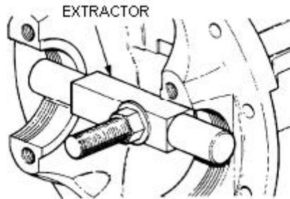
**Figure 234 Removing the Pinion Shaft Inner Bearing Cup**
