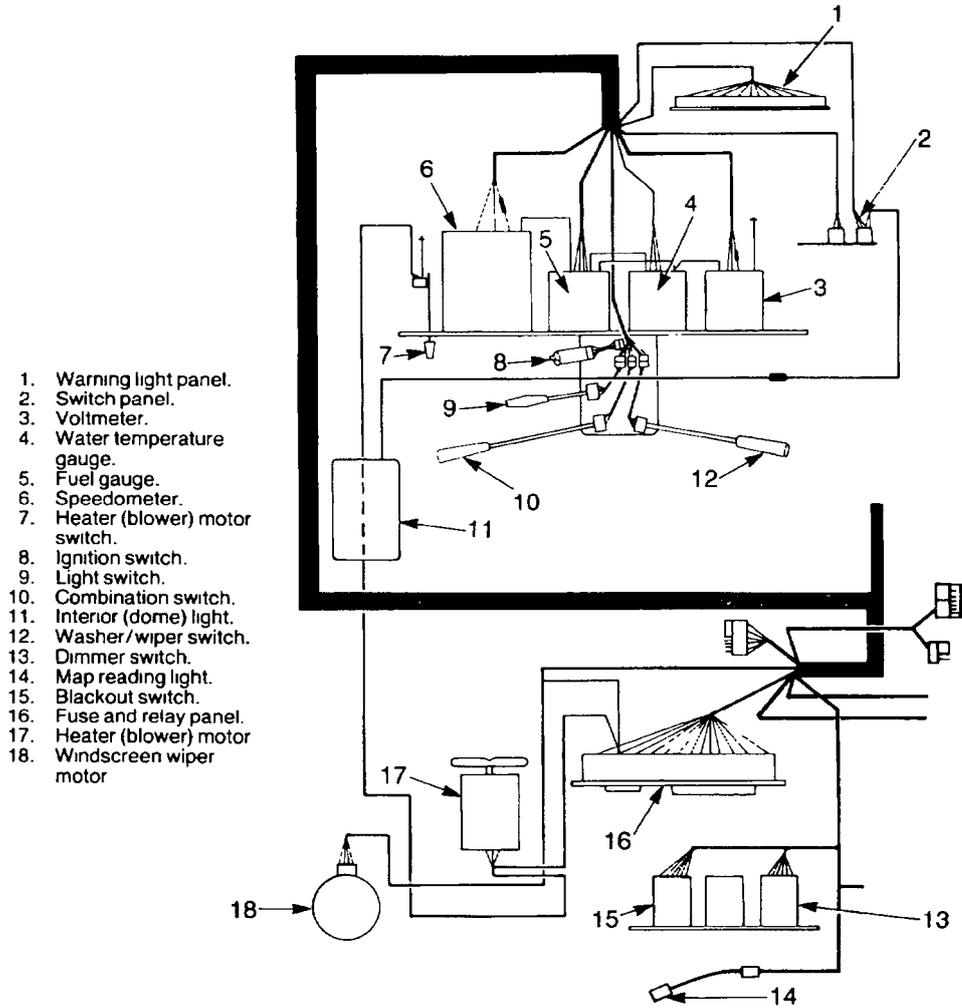
Figure 309 Cab Wiring
