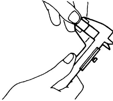
**Figure 299 Measuring the Vacuum Pump Vanes**
