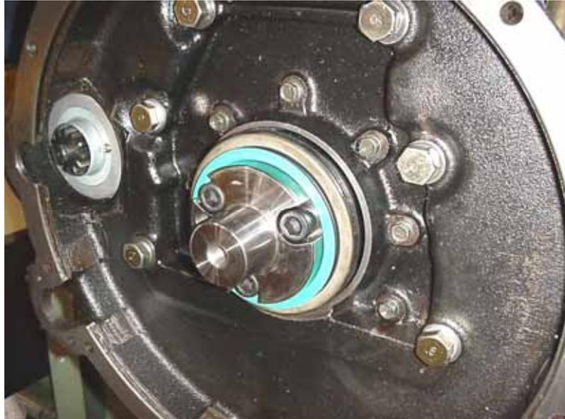
**Figure 48 Rear Crankshaft Oil Seal Located on Crank Plate Ready for Installation**
