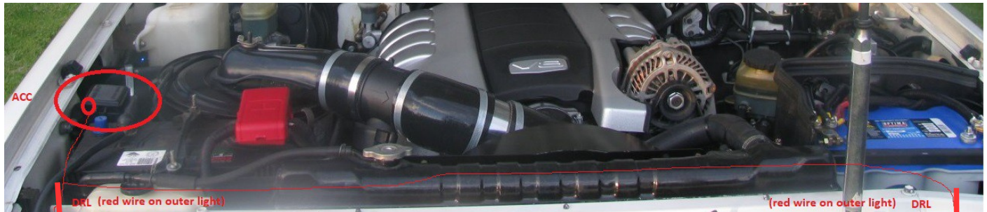
Illustration 2: Connect the RED Wire spade connectors to the ACC terminal in the box on drivers side to terminal labelled ACC.
