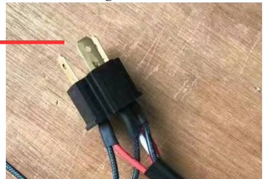
Illustration 3: This MALE plug . Plugs into the OUTER light H4 Connector where you removed your old lights from the OE car wiring harness.
