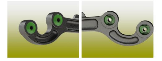
1./ **BEFORE Lifting the vehicle.** Mark the *horizontal* position next to all 4 bushes on the arms for alignment. Inside and outside.
